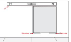
Securely fasten the vanity to the wall through back of vanity with appropriate screws/bolts at TOP and BOTTOM of cabinet. Fix the cabinet through the top left and right hand brackets. For the bottom start the fixing points no further than 100mm from each end of the cabinet and no higher than 50mm from the base panel.
