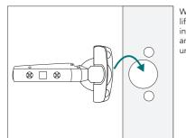
With top cover plate lifted, place hinge into position on door and insert into holes until flush.
