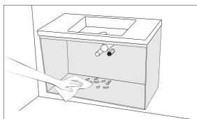
Clean all building residue from the cabinet. Dry any spillage or leakage of water on or inside the cabinet during installation.
