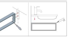
Fix bracket with the 10Gx50 screws provided.
