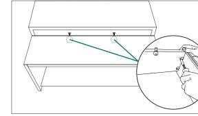
Carefully lay vanity unit on its back on a flat surface. Using the pre-drilled holes at the base of the unit as a guide, insert the cam-locks at the top of the kicboard and fasten to vanity unit.
