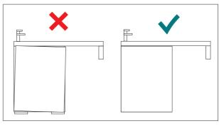
Install drawers and doors back onto cabinet and make adjusments to align the doors and drawers correctly.
