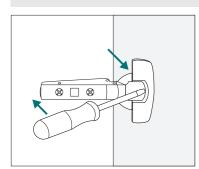
Once you have removed door from the cabinet, using a flat head screw driver, lift and release the
