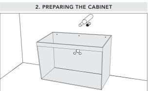
Remove door. Measure correct plumbing loctions and drill holes for plumbing in the back panel and/or base of the cabinet with an appropriate sized hole saw. Pre-drill screw locations for fastening to wall as per 'Step 4'.
