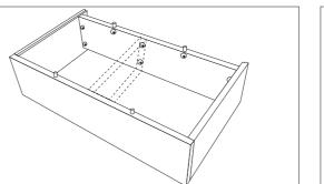
For larger units (1200mm and bigger), insert the centre support panel supplied and secure all cams.
