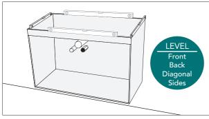
Position the vanity over the pipes in the correct position and fix with a single screw in centre of vanity to hold in place.
