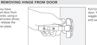
Pull hinge up and out from door. You may need to wiggle the hinge to loosen and use a little force.
