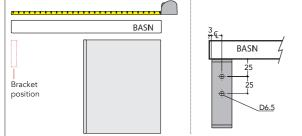
Measure basin length to mark the position of the bracket. Mark position of the holes and then drill two 3mm holes.
