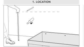
After completing the Prior to Installation Checklist on page 2, mark the position of the top of the vanity. Don't forget to factor in the top/ basin thickness to get the correct height.
