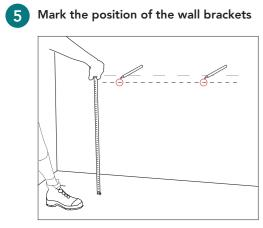
Mark the bracket positions on the wall. All three holes in each bracket should fall within the support beam.
