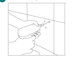
Pre-drill into the wall through each of the hole locations in the wall bracket (3 per bracket). Be sure to use an appropriate drill bit for your wall covering (tiles etc).
