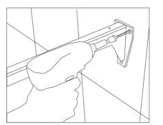
Secure each bracket to the wall using an appropriate screw/bolt.
