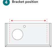
Measure the bracket position on the underside of the bench, making sure to leave enough room for the basin, waste and plumbing.
