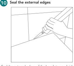
Seal the external edges of the bench top and sides to the wall with a neutral cure silicone.
